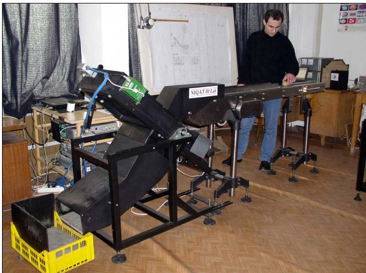
**Fig. 3** – Experimental model of the system NIQAT01Lab for classification in real time of potato tubers by internal diseases and defects
