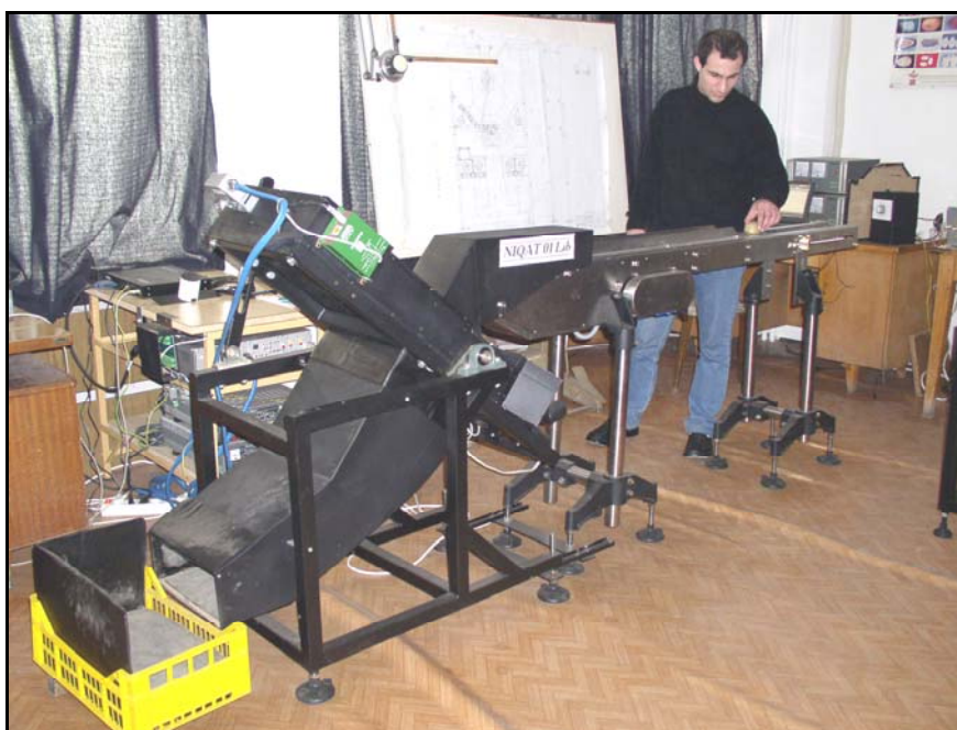
Fig. 2 - NIQATLAB model, which classifies potatoes according to internal defects and the influence of skin (peel) is eliminated (RCSAS- Plovdiv at NCAS)
